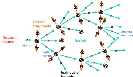
Figure 3: Nuclear fission chain reaction.
